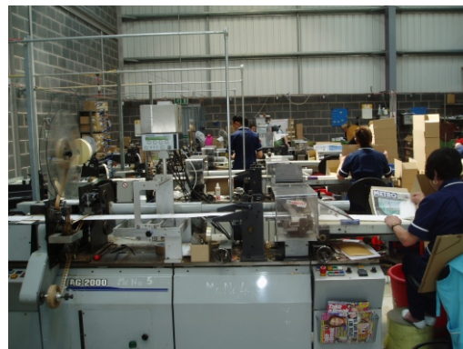
Our Tag machines cut & washer Up to 10,000 tags per hour.
